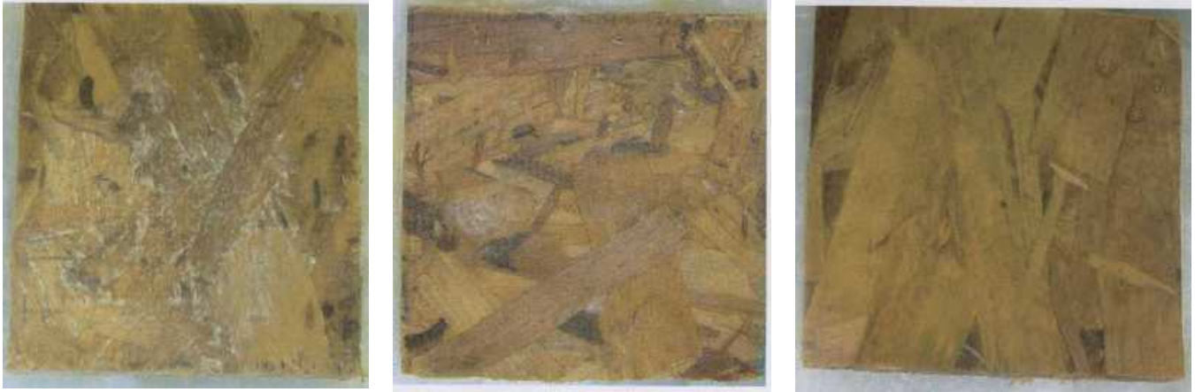
Picture 1: 60 days after mold treatment. Left: Control | Middle: Bleach | Right: PURStrike®
